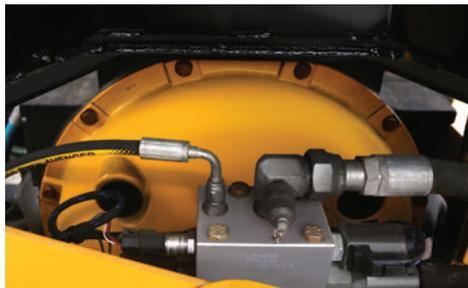
**SELF-ADJUSTING CLUTCH.** Automatic, push-button clutch provides consistent engagement every time — helping to prolong clutch life, lower maintenance costs and reduce operator error.
