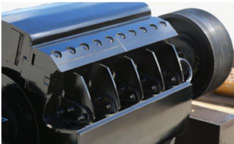
**EASIER KNIFE SETUP WITH FLEXIBLE CHIP SIZING.** Microdrum design improves productivity over higher horsepower models. Knife position is set with two bolts—no babbiting needed, making jobsite knife changing easier. Adjustable bite size in 1/8" (.3 cm) increments, up to 5/8" (1.6 cm).
