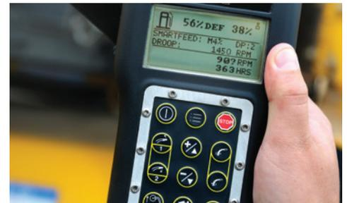
**CONVENIENT REMOTE CONTROL.** ACS control system designed specifically for this machine allows operators to engage/disengage clutch and control trip meter, Ecolde™ engine control system and work lights from the remote.
