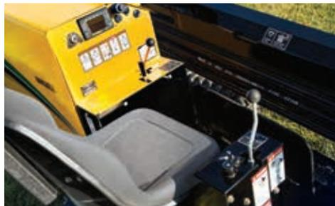
**OPERATOR'S STATION.** The D6x6 has dual axis control valves. Vise controls are integrated into the right- and left- hand joysticks. With this design, the operator's hands do not have to leave the joystick to run the controls.
