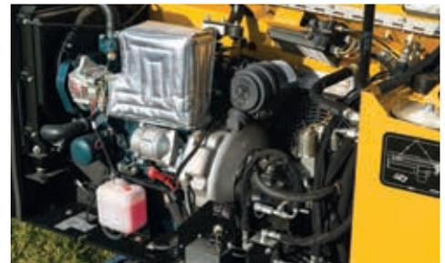
**SERVICEABILITY.** A full-length hood opens to expose the engine and hydraulics for easier maintenance and service.
