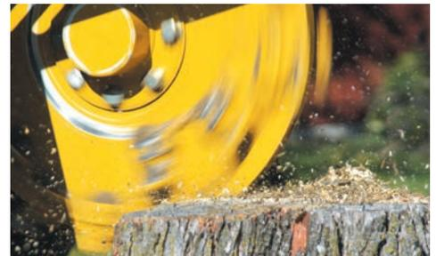
**PATENTED YELLOW JACKET™ CUTTER SYSTEM.** The Vermeer-exclusive Yellow Jacket cutter system is designed to provide faster, easier serviceability, as well as extended pocket and tooth life.
