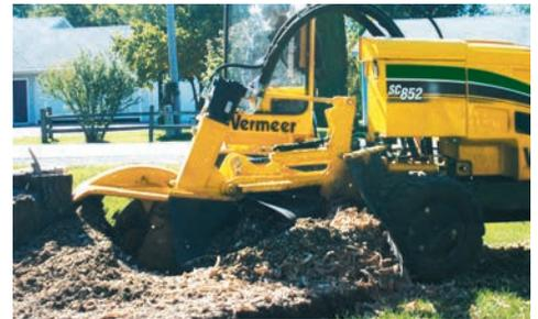
**CHIP CONTAINMENT.** Ground clearance allows plenty of room for chip containment, while the rounded chip blade moves chips around the jobsite easily, reducing the need for manual chip moving. A wide wheel base provides stability; a differential lock on the 4WD system can be disengaged for tight turning.
