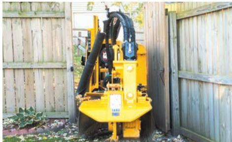
**COMPACT FOOTPRINT.** Front-mounted controls offer maneuverability in confined spaces by allowing the operator to walk in-line with the machine.
