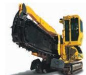
**ELEVATING ROPM CAB.** The elevating rollover protective module cab features LEXAN glass, filtered and pressurized air, heating and air-conditioning. The cab's vantage point allows a virtually unrestricted view of the boom, trench and conveyor.
