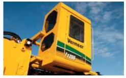
**ELEVATING ENCLOSED CAB.** The elevating cab allows superior visibility and added comfort with the air ride seat. The sealed cab has selfcontained heating and air conditioning with sound attenuating foam. It is also a rollover protective module (ROPM) and provides falling object protection (FOPS).
