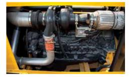
**ENGINE POWER.** The FPT Tier 4 Final engine provides 515 hp (384 kW) of power to meet your jobsite demands.
