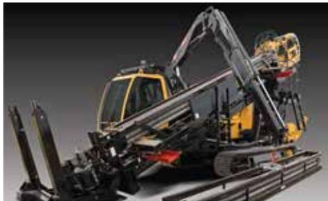
**OPTIONAL ONBOARD CRANE.** Choose the optional onboard knuckleboom style crane to reduce the amount of support equipment needed onsite.
