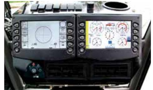
**MONITOR YOUR DRILLING ACTIVITY.** Standard dual large, color LCD monitors offer visibility to machine information and DCI locator information.
