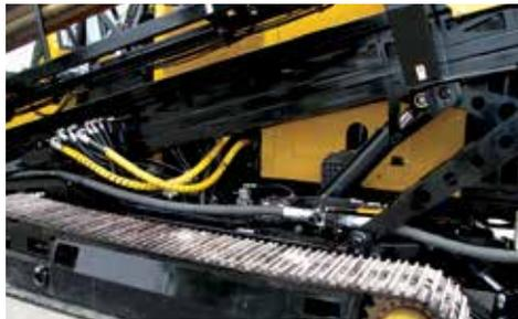
**INCREASE YOUR RANGE.** Unique four-bar linkage rack and additional pads allow operators to set up entry angles ranging from 12 - 24° (15' rod option) and 8 - 24° (20' rod option) increasing range attainable with tracks fully on ground.
