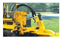
**DIRECT DRIVE.** Direct drive hydrostatic pump and gearbox eliminates clutch and belt-drive maintenance. Cutter wheel stopping time is reduced with no-maintenance hydrostatic braking.
