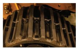
QUAD TRACK SYSTEM. The guad track system offers improved flotation, reduced surface damage and increased tractive effort. Four-wheel steer and crab steering are functional with both quad track and tire options.
