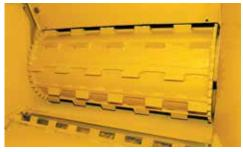
LOWER FEED ROLLER. The lower feed roller is offset from the upper feed roller by 10.75" (27.3 cm). Material is easily pulled to the upper feed roller, so there is less need to manually raise the upper feed roller for larger diameter material.
